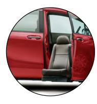
**BRAUNABILITY TURNY EVO SWIVEL SEAT** is the #1 selling handicap vehicle transfer seat for SUVs, trucks, and vans that moves completely outside the vehicle and lowers it down to your desired level. This makes it easier for you to sit down or transfer from a wheelchair.
