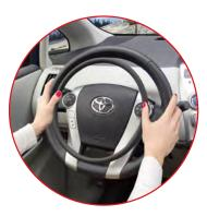
Hand controls, allowing the driver to operate the vehicle's throttle and brakes with only their hands, are common adaptive equipment options for drivers with limited mobility.
